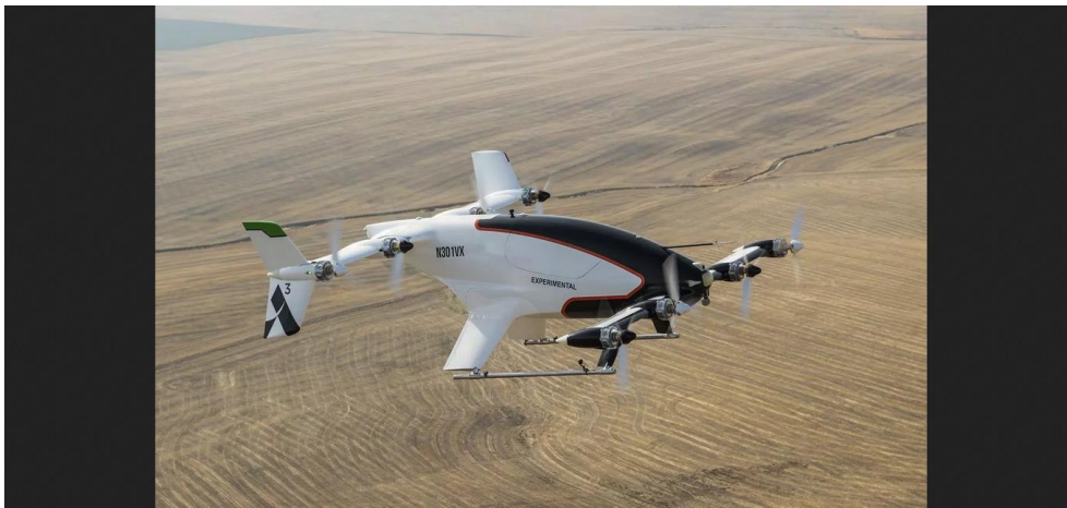
Figure 7 : Envisioning future urban air mobility. From sketch to reality of Airbus Vahana eVTOL demonstrator.
